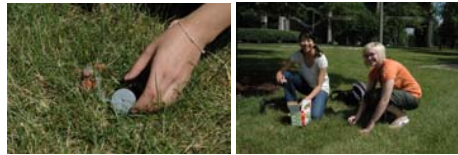
Figure 2. Students buried the canisters into the ground. Squirrels, upon finding the nuts, may collect, eat or hide them away. As the squirrel moves the nut, the spool remains anchored in the container, and the thread plays out.
