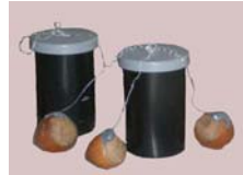
Figure 1. Nylon spools of thread are attached to hazelnuts with epoxy, and three spools (500 m each) are placed inside each plastic canister.
